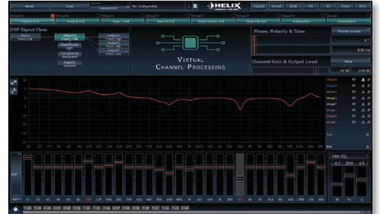
The setup of the virtual channels is similar to that of the output channels, only without crossovers. The virtual front EQ and FX front processing then affect all output channels routed from there
