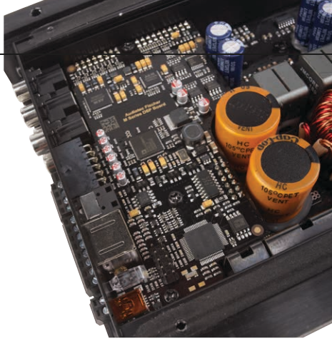
The DSP board of the M FOUR DSP replaces the analog input board of the M FOUR
